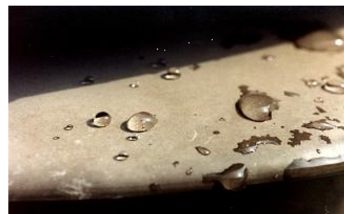
Fig. 6: Water droplets on a pollution layer on a SIR shed [2]
